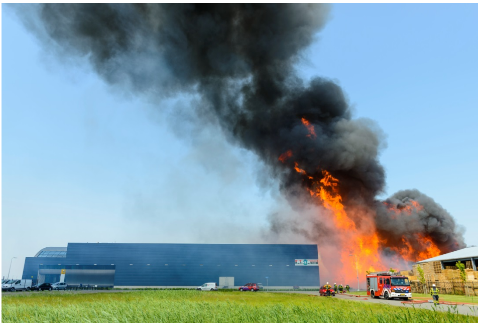
Figure 7 Flame length of up to 51m (Source: Sjoerd van der Wal Fotografie)
