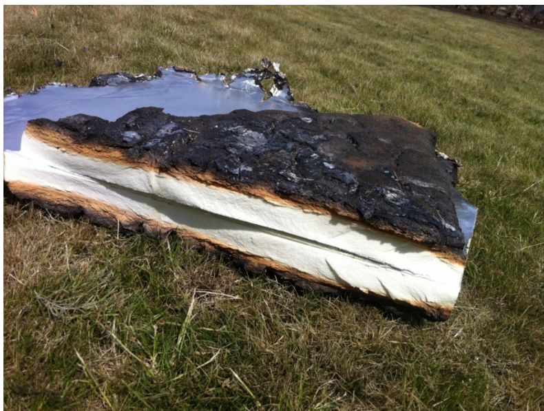
Figure 17 Charring and discolouration of the insulation (Source: Kingspan Insulation)
